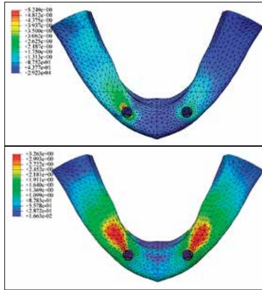
Fig. 4. Stress distribution pattern in ball attachment model when load applied. *Top.* Unilateral. *Bottom.* Bilateral.<sup>24</sup>
