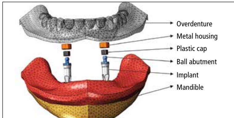
Fig. 1. Computerized mesh modeling showing jaw and overdenture with ball attachment.<sup>24</sup>
