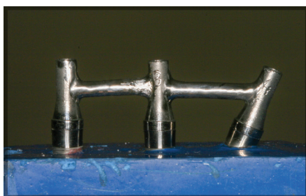
Fig 2. Metal framework used to measure the marginal gap.
