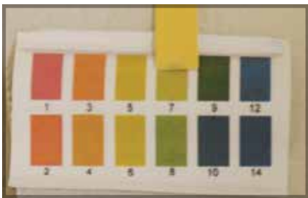
Fig 4. After the pH measuring paper has contacted the bleaching gel, the color on the edge of the paper is compared to the pH scale; the closest color indicates the approximate pH value of the gel.
