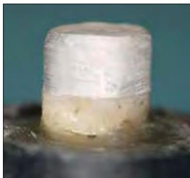
Fig. 5. A Tytin specimen with a 1 mm bevel at the axial-occlusal line angle.
