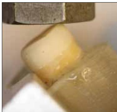
Fig. 6. A FluoroCore 2 specimen in the universal testing machine.
