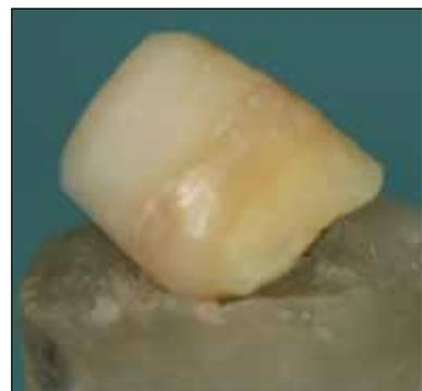
Fig. 7. Root fracture of a FluoroCore 2 specimen retained by pins and Optibond Solo Plus with BondLink. The core foundation remained intact.
